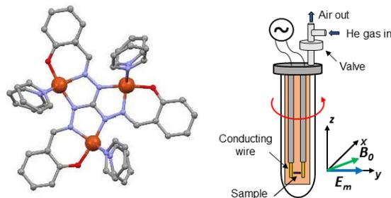
Fig. 1 Left: the molecular structure of the spin-frustrated Cu<sub>3</sub>, with a ground state  $S=1/2$ . Right: schematic view of the modified version of the sample holder used for the EFM-EPR measurements. The orientations of the static magnetic field ( $B_0$ ), and the electric field ( $E_m$ ) are shown.  $E_m$  is obtained by applying an alternating voltage  $V = V_0 \cos(\omega t)$ , with  $V_0 = 170$  V over a distance of 1.5 mm, and  $\omega = 2\pi \times 30$  kHz.
